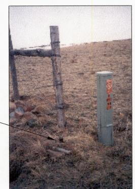
TELEPHONE PEDESTAL-2.0.\* PK NAIL IN POST (TYP.) -FOUND BRASS CAP IN A IRON PIPE. 23 1974
